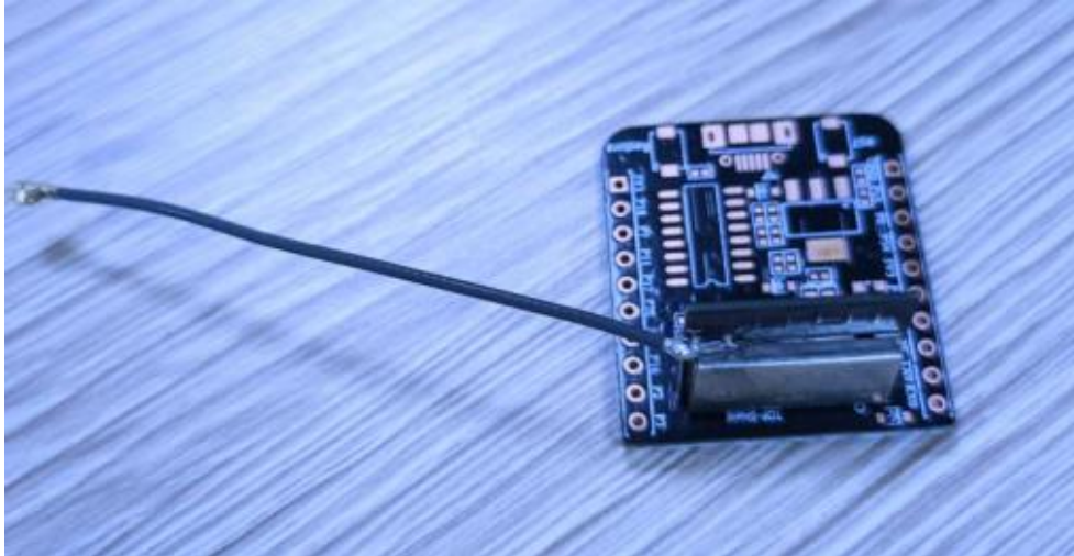
Figure 8 Schematic diagram of the antenna test prototype
